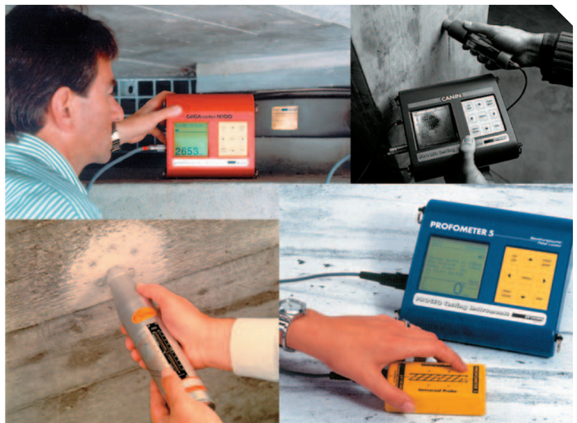
Bridge inspection with Proceq testing instruments like SCHMIDT, PROFOMETER, CANIN
