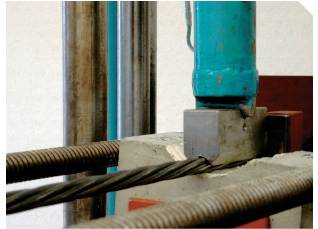
Plastic duct under wear resistance compliance test
